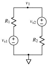
Use the node-voltage method to find a formula for  $v_1$ . Write your answer as a sum of a voltage divider for  $v_{s1}$  and a voltage divider for  $v_{s2}$ .
