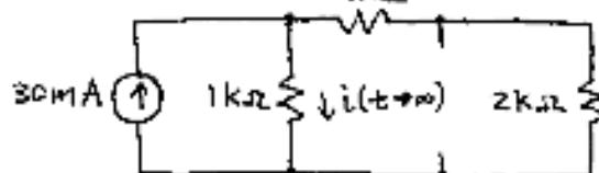
We have a current divider with  $1k\Omega$  on left and  $1k\Omega + 2k\Omega = 3k\Omega$  on right.
