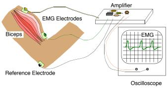
Figure 1. System for measuring an electromyogram.
