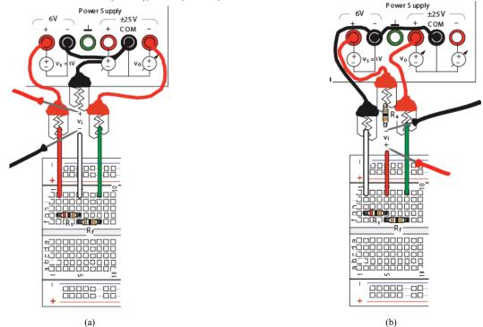
Figure 6. Protoboard layouts for modeling op-amp circuits and measuring  $v_i$ : (a) negative-gain op-amp circuit, (b) positive-gain op-amp circuit.
