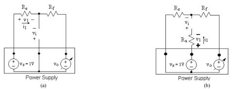
Figure 4. Circuits for modeling op-amp circuits: (a) negative-gain op-amp circuit, (b) positive-gain op-amp circuit.
