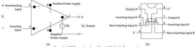
Figure 5. LF353 operational amplifier: (a) Model, (b) Pins on package.
