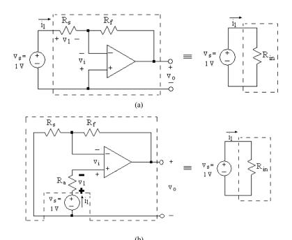
(b) Figure 8. Input resistance Rin for pre-amp circuits: (a) negative-gain circuit (b) positive-gain circuit
