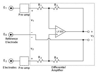
Figure 10. Schematic diagram of electromyogram circuit.
