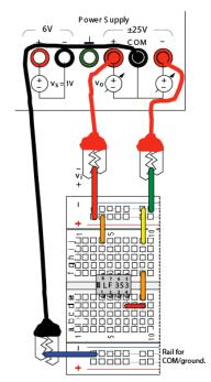
Figure 9. Protoboard and power-supply connections for power to op-amp.
