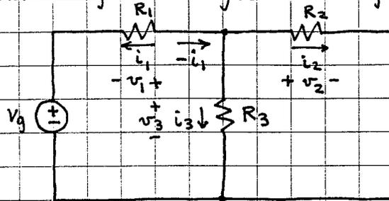
Total current,  $-i_1 = \frac{V_g}{R_1 + R_2 \parallel R_3}$
