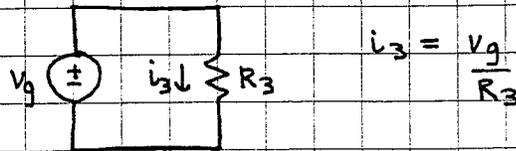
Our formula with  $R_1 = 0$ :  $i_3 = \frac{V_g R_2}{R_2 R_3} = \frac{V_g}{R_3}$
