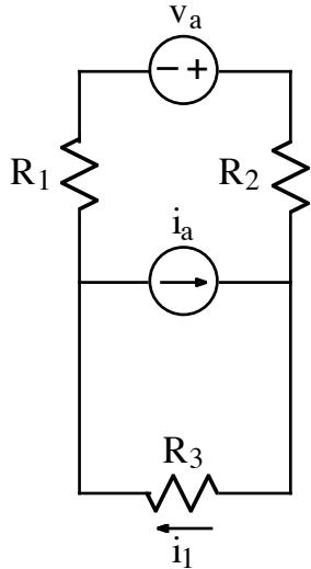
Derive an expression for  $i_1$ . The expression must not contain more than the circuit parameters  $v_a$ ,  $i_a$ ,  $R_1$ ,  $R_2$ , and  $R_3$ .
