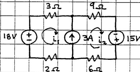
Use mesh-current method to find total pwr dissipated by circuit.
