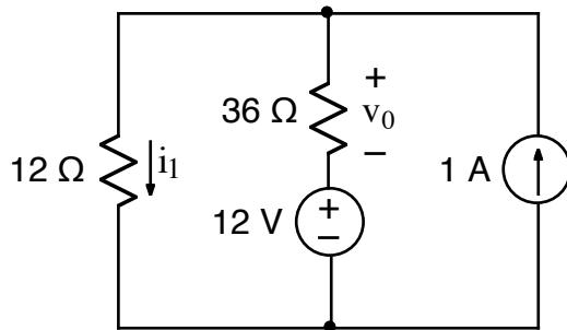
Use the node-voltage method to find  $i_1$  and  $v_0$ .
