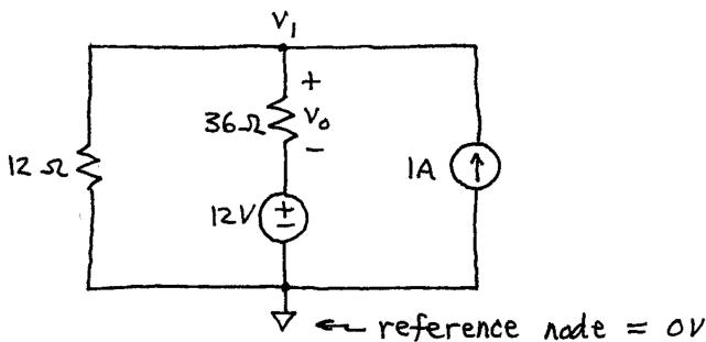
The  $-$  sign of all voltage measurements is at the reference node. Thus,  $v_1$  is the  $v$ -drop from the top node to the reference node.
