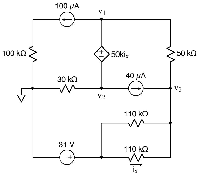
Use the node-voltage method to find  $v_1$ ,  $v_2$ , and  $v_3$ .
