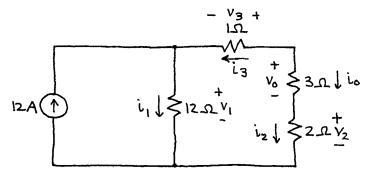
Now we write eghs for voltage loops. We try to write v-loop eghs for inner loops, but we avoid loops that include a current source. (The reason we do so is to avoid defining a new variable that requires another egh.) In this problem, there is only one v-loop without a current source. Going around the inner loop on the right side in a clockwise direction and using the sign where we exit a component, we have
