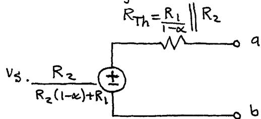
Note: For the first part of this problem, when we calculate  $V_{Th}$ , we may use an equivalent resistance in place of the dependent source.
