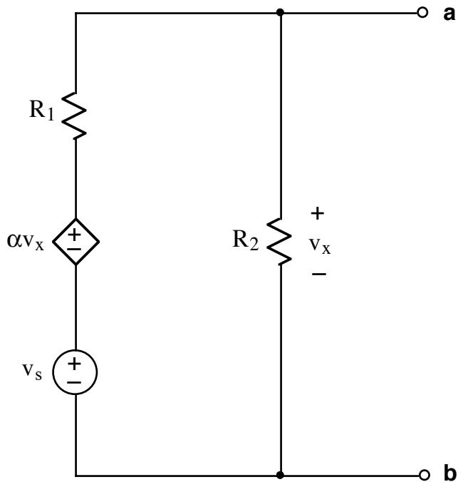
Find the Thevenin equivalent circuit at terminals a-b.  $v_x$  must not appear in your solution. **Hint:** Use the node voltage method. **Note:**  $0 < \alpha < 1$ .
