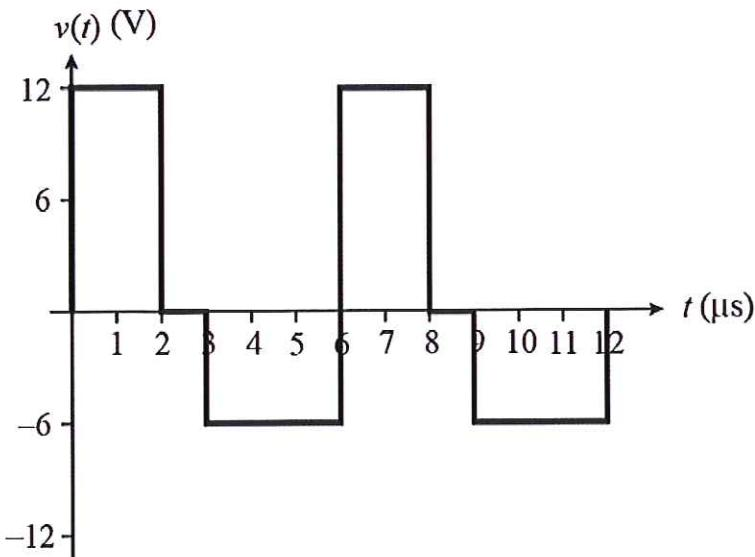
A portion of a repetitive waveform,  $v(t)$ , is shown above.
