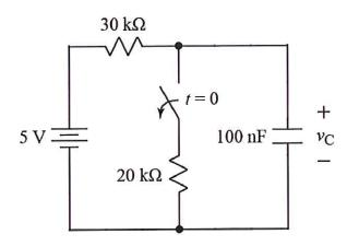
The switch is closed for a long time before opening at t = 0.
