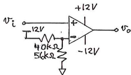
We want  $v_- = 7V$ . Use V-divider:  $v_- = 12V \cdot \frac{56k\Omega}{96k\Omega}$
