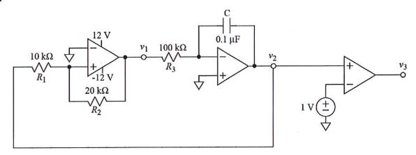
The above circuit is from Lab 4, but some of the component values have been changed. Note that voltage  $v_2$  is a triangle waveform, and  $v_3$  is a Pulse-Width Modulation (PWM) waveform.
