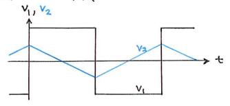
$v_1$  switches from + to - when  $v_2$  (triangle wave shown above) causes  $v_+ = 0v = v_-$  for first op-amp.
