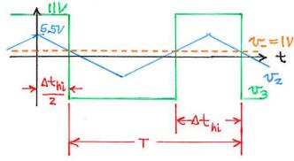
The duty cycle is  $\Delta t_{hi}/T$ . T=20ms from (b).
