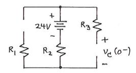
No current flows, so R's all have OV drops. From V-100p around center and right side,  $V_{c}(0^{-}) = 24V$ .
