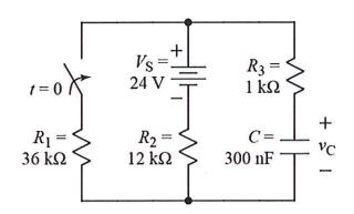
The switch has been open for a long time and is closed at t = 0.
