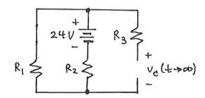
There is no current in  $R_3$  and no V-drop across  $R_3$ . So  $V_c$  is the same as the V across the center branch and the same as the V across  $R_1$ . We use the V-divider formula to find the V-drop across  $R_1$ .
