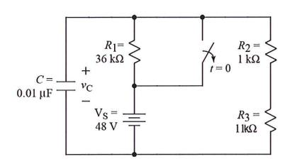
The switch has been closed for a long time and is opened at t = 0.
