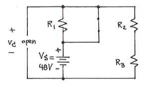
If we follow wires from the 48V source, we find they are leading directly to the C. So  $V_{\rm C}(0^-) = V_{\rm S} = 78V$ , and  $V_{\rm C}(0^+) = V_{\rm C}(0^-)$ .
