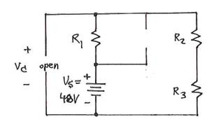
To find  $R_{Th}$  for time constant  $\mathcal{C} = R_{Th} \mathcal{C}$ , we look in from the terminals where  $\mathcal{C}$  is connected and turn off  $V_{\vec{S}}$  (= wire).
