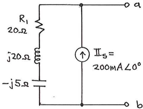
$V_{Th} = V_{ab}$  in above circuit.  $I_s$  flows thru  $R_1$ ,  $Z_L$  and  $Z_C$ , creating voltage drop  $V_{ab} = V_{Th}$ .
