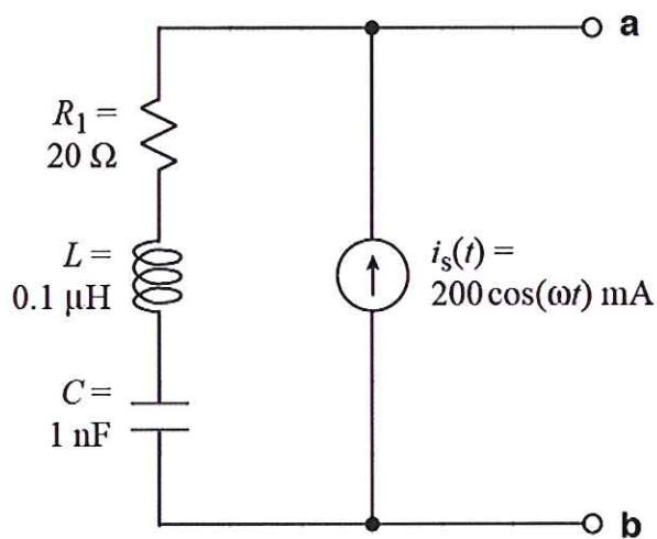
Find the Thevenin equivalent of the above circuit in the frequency domain. That is, find the values of phasor  $\mathbf{V}_{Th}$  and impedance  $z_{Th}$  in the equivalent circuit below.
