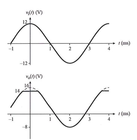
Using op-amps, power supplies, and resistors, draw a circuit to produce  $v_0(t)$  from  $v_i(t)$ . (Assume you have a function generator that produces  $v_i(t)$  for you to use.) Show all relevant information in your circuit, including positive and negative power supply voltages for op-amps. You may use only two power supplies in your design. You must generate any other voltages you need from those two power supplies, (for example by using a voltage-divider).
