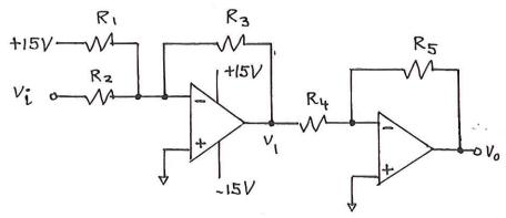
For first stage,  $V_1 = -15V \frac{R_3}{R_1} - V_1 \frac{R_3}{R_2}$ .
