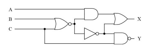
Complete the truth table, below, for the logic circuit above. (Note that you must fill in some missing input values in the table, too.)
