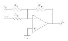
5.) Redraw the same circuit as problem 4, only now follow it with an inverting amp with a gain of 1. Say  $R_3 = R_4 = 10 \text{ k}\Omega$  for the second op-amp.
