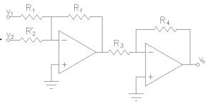
6.) Draw a differential amplifier. Choose an  $R_{in}$  value. Make  $R_f$  12 times bigger than  $R_{in}$ . Say  $R_{in}$  = 10 k $\Omega$  and  $R_f$  = 120 k $\Omega$ .
