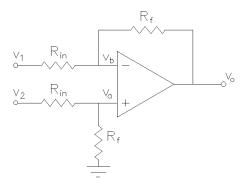
7.) Just choose the two resistor values to be equal, so the voltage at the inverting input pin will be 5 V. Now, anytime the voltage on the noninverting pin is above 5 V the output will be high (~8 V) and anytime the voltage on the noninverting pin is below 5 V the output will be low (~2 V).
