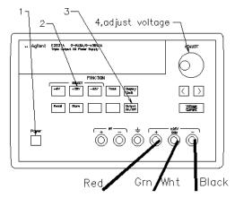
the same voltage value as) the + output. Adjust the + output to 6 V. Now the power supply will output  $\pm$  6 V. Turn off the power switch on the servo. Now hook up the servo as shown. (Turn the outputs off again while connecting.) Watch out, remember the HP/Agilent's + connection and it's – connection are *both* red, – is on the right side of ground and + is on the left.
