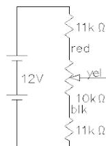
Measure the voltage at the two extremes of the potentiometer rotation. The potentiometer rotates about  $270^\circ$ .  $K_p$  is the change in volts per change in angle. Determine  $K_p$  as volts/deg and as volts/rad.
