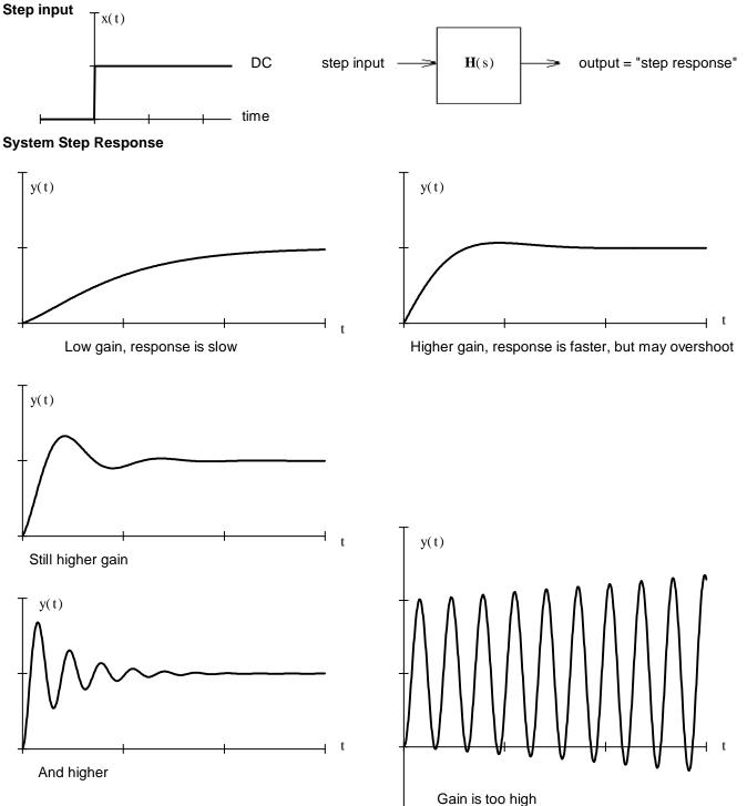
The step response of a system is the output when the input is a step (DC which starts at time-zero). Step input  $-\pi$  (C)
