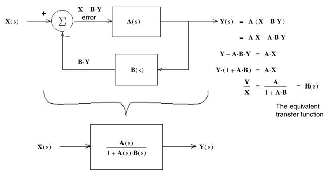
This is called a "closed loop" system, whereas a a system without feedback is called "open loop". The term "open loop" is often used to describe a system that is out of control.
