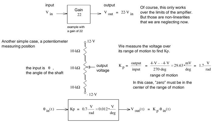
Nice... too bad it works for so few things in the time domain! Simple voltage dividers, amplifiers, and not much else. In real electrical systems there are always capacitance and inductance.
