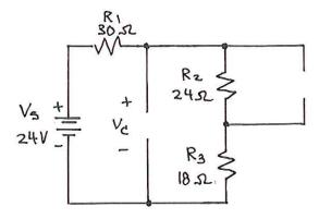
We find  $V_c(0^-) = V$  across  $R_2 + R_3$  by using a V-divider.
