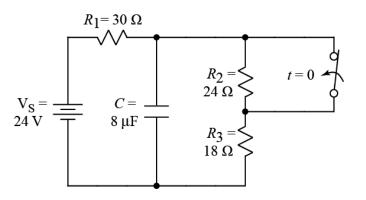
The switch has been open for a long time and is closed (as shown) at t = 0.
