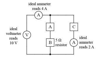
If box A contains a resistor, find the value of that resistor.
