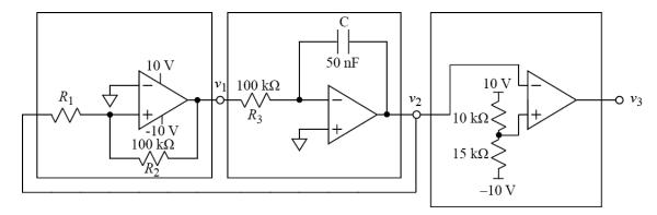
The above circuit is from Lab 4, but some of the component values have been changed.
