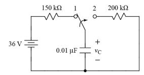
After being on side 1 for a long time, the switch moves from side 1 to side 2 at t = 0.
