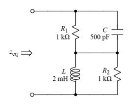
Find the numerical value of the equivalent impedance,  $z_{eq}$ , for the circuit. Frequency  $\omega = 1$  Mr/s. Express your answer in both rectangular and polar form.
