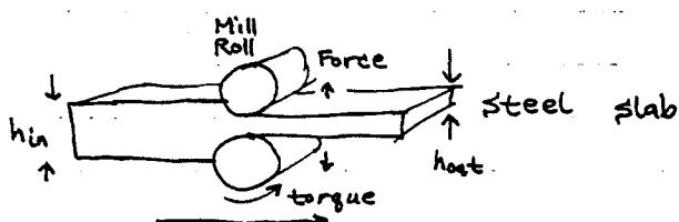
When we roll a slab, we can calculate the torque and force required. The equation for force is (note: there are probably small errors in these eqns):
