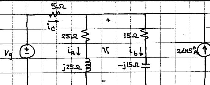
Given  $I_b = 5 \angle 45^\circ A$  is phasor for current  $i_b$ .
