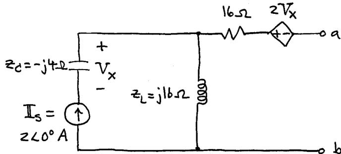
b)  $V_{Th} = V_{ab}$  open circuit.
