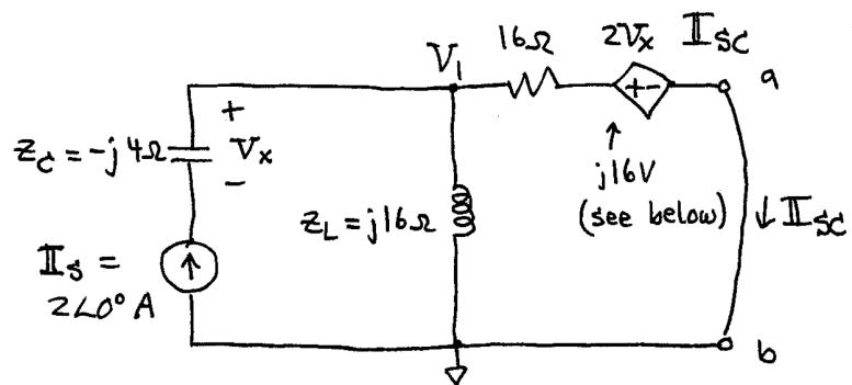
Since  $C$  is in series with current source, we have  $V_x = -I_s z_C = j8V$  as before.
