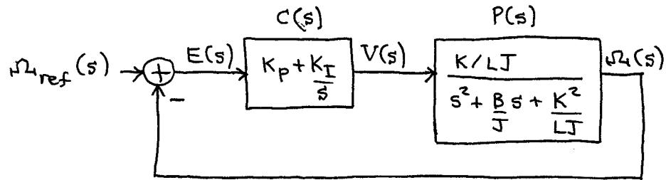
b) From eqns of system or from block diagram
