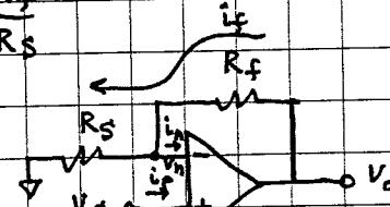
$$\text{input resistance} = \frac{V_s}{i_s} = \frac{V_s}{i_f} = \frac{V_s}{0} = \infty$$
