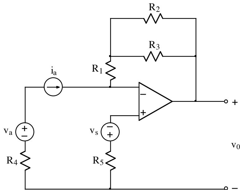
The op-amp operates in the linear mode. Using an appropriate model of the op amp, derive an expression for  $v_0$  in terms of not more than  $v_a$ ,  $v_s$ ,  $i_a$ ,  $R_1$ ,  $R_2$ ,  $R_3$ ,  $R_4$  and  $R_5$ .
