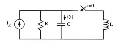
After being open for a long time, the switch closes at t = 0. The inductor carries no current at time  $t = 0^-$ .
