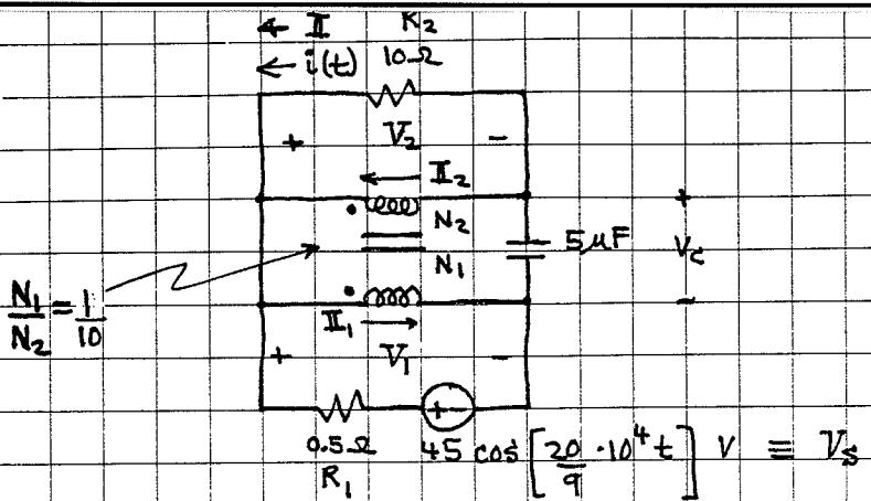
Given an ideal transformer in the above circuit, calculate  $i(t)$ .
