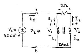
Note: The + signs for  $V_1$  and  $V_2$  are at the dots. In flows into the dot, and II 2 flows out of the dot.
