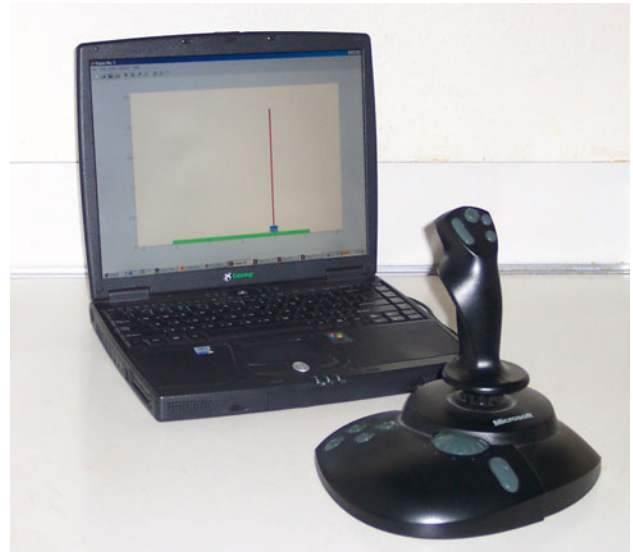
Figure 1: Controlling a simulated inverted pendulum through a joystick
