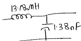
Design a L-Network to match a 100 ohm source to a 1000 ohm load at 100 MHz. Assume DC voltage must be transmitted.
