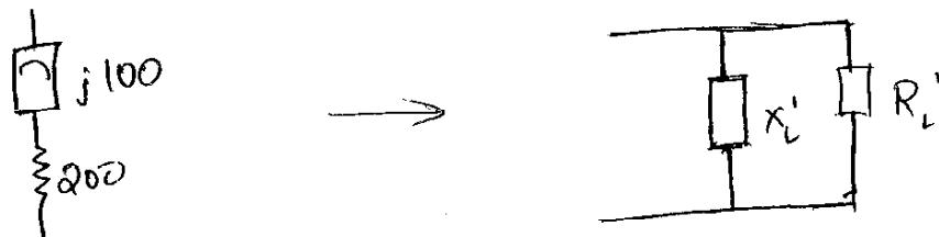
$$R_L' = \frac{R_L^2 + X_L^2}{R_L} = \frac{(200)^2 + (100)^2}{200} = 250 \Omega$$
