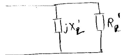
$$R_L' = \frac{R_L^2 + X_L^2}{R_L} = 97.16\Omega \quad X_L' = \frac{R_L' R_L}{X_L} = 168.87\Omega$$
