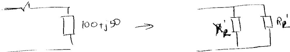
$$R_L' = \frac{R_L^2 + X_L^2}{R_L} = \frac{(100)^2 + (50)^2}{100} = 125 \Omega$$
