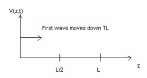
Velocity of wave  $vp = 1/sqrt(\epsilon\mu)$ Wave moves down TL with no reflections until it reaches the load ... Time to reach load: T = L / vp
