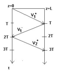
$V(L/2,3T) = V_1^+ + V_1^- + V_2^+$
