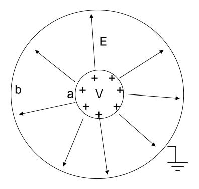
For 2-conductor transmission line, V is voltage between the conductors  $V = \int_{+}^{-} \overline{E} \bullet d\ell = \int_{a}^{b} \frac{V}{r \ln(b/a)} \bullet dr = V \frac{\ln(b/a)}{\ln(b/a)} = V$ I is current flowing on the positive conductor
