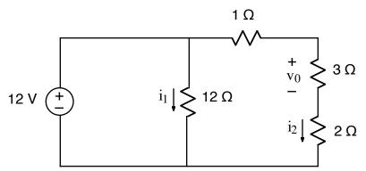
Using the passive sign convention, complete the labeling of all currents and voltages for the resistors in the above circuit.
