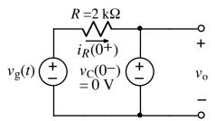
We find the current in the R by taking the voltage drop across the R and using Ohm's law:
