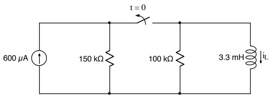
After being closed for a long time, the switch opens at t = 0. Find  $i_L(t)$  for t > 0. Hint: use a Thevenin equivalent for the circuit to the left of the inductor.
