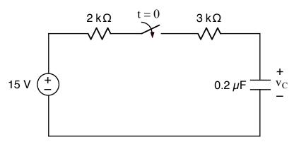
After being open for a long time, the switch closes at t=0.  $v_C(t=0^-)=0V$ . Find  $v_C(t)$  for t>0.
