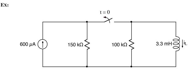
After being closed for a long time, the switch opens at t = 0. Find  $i_L(t)$  for t > 0.
