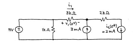
A current summation at the node shown as a large dot gives the current thru the 3kQ resistor:
