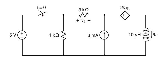
After being open for a long time, the switch closes at t = 0. Find  $v_1(t)$  for t > 0.
