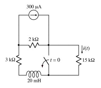
After being closed for a long time, the switch opens at t = 0.
