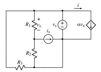
Using superposition, derive an expression for *i* that contains no circuit quantities other than  $i_s$ ,  $v_s$ ,  $R_1$ ,  $R_2$ ,  $R_3$ , and  $\alpha$ .
