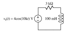
a) Find time-domain expressions for the waveforms of the voltages across the R and L in the above circuit.
