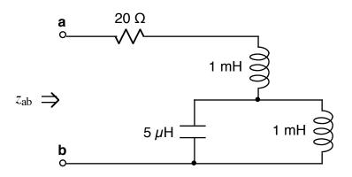
Find a frequency,  $\omega$ , that causes  $z_{ab}$  to be real, (i.e., imaginary part equals zero). Sol'n:  $z_{ab} = 20 \ r + z_{LI} + z_{CI} \| z_{L2}$
